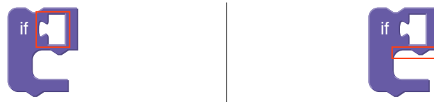
Figure 7.4: If block that highlights the usage of an input value block (left) as its first argument (condition of the if statement) and a statement input (right) as its second argument (body of the if statement).
